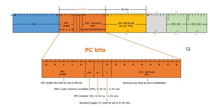
The Tag shall implement the StoredCRC by first calculating a CRC-16 over the StoredPC and the EPC specified by the length (L) bits in the StoredPC, and then storing the thus-computed StoredCRC into EPC memory 00h to 0Fh. The Tag shall calculate the StoredCRC on word boundaries, shall deassert all Tag-computed StoredPC bit values (XI and UMI if Tag-computed) when performing the calculation, and shall omit XPC W1 and XPC W2 from the calculation.
