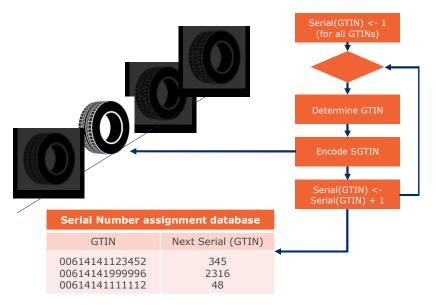
The serial number assignment database keeps track of the next available serial number for each GTIN being manufactured. As in the previous case, it is imperative that this information is carefully backed up.
