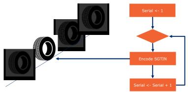
In this example, the first instance of the tire receives serial number 1, the second receives serial number 2, and so on. If the full 38-bit serial number available in the SGTIN-96 RFID tag is consumed in this way, there is capacity to serialize  $2^{38} = 274,877,906,944$  instances of a tire (GTIN) without duplications.
