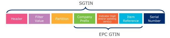
**NOTE:** Indicator Digit is only used for GTIN-14. As the creation of SGTIN-96 numbers for tires is based only on GTIN-12 and GTIN-13 constructs, Indicator Digit will no longer be considered in the rest of the document.
