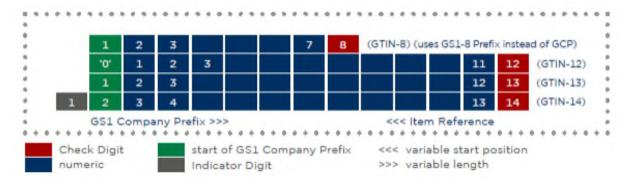
GTIN-8 are mainly used for very small products for which the space is restricted. GTIN-14 are used when indicator digit is required for packaging level identification. Therefore, both GTIN-8 and GTIN-14 shall not be used for unique tire identification.
