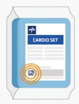
The tag, placed on each tray, features an antenna that transmits a signal with a unique ID to identify the specific pack being used. This tag provides the following product data with **GS1 standard codification**:
